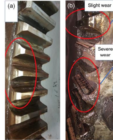
Fig. 17 Wear of gears in a wind turbine.
